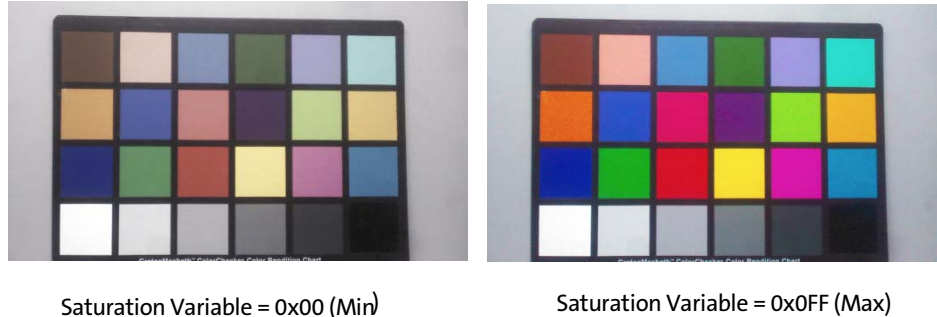
Figure 44: Saturation Variable Min and Max
