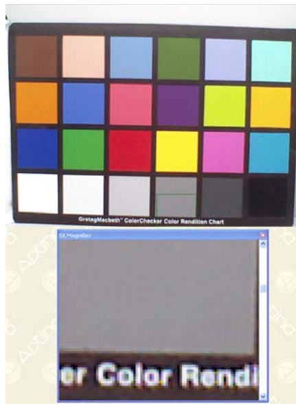
Figure 48: Sharpness Threshold = 0xFF (Max)
