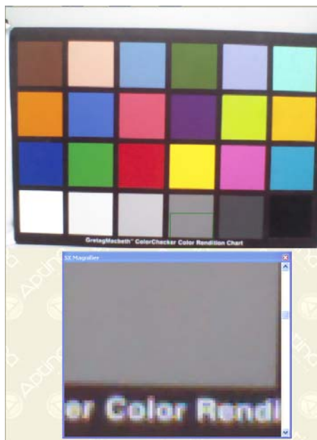
Figure 48: Sharpness Threshold = 0xFF (Max)
