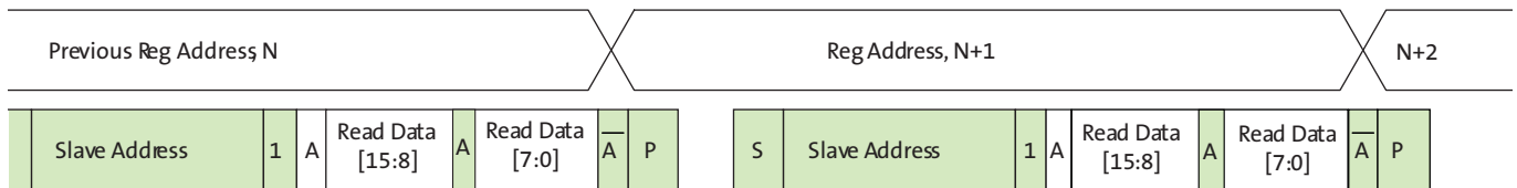
Figure 23: Single Read from Current Location
