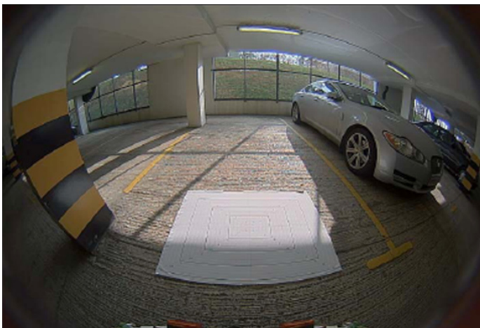
Distorted Image from Wide Angle Lens
