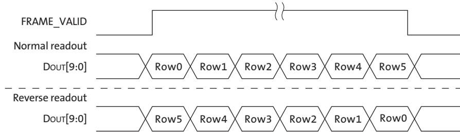
The MT9V113 sensor core supports subsampling with skipping to increase the frame rate. The proper image output size and cropped size must be programmed before enabling subsampling mode. Figure 10 shows the readout with 2X skipping.
