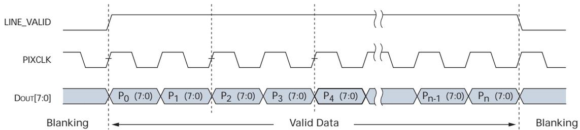
**Figure 4: Row Timing, FV, and LV Signals**
