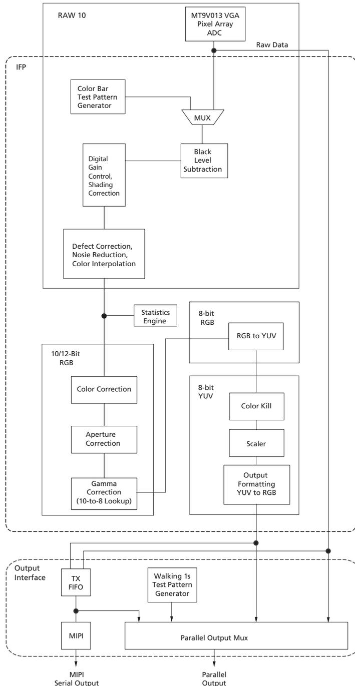
For normal operation of the MT9V113, streams of raw image data from the sensor core are continuously fed into the color pipeline. The MT9V113 features an automatic color bar test pattern generation function to emulate sensor images as shown in Figure 16. The color bar test pattern is fed to the IFP for testing the image pipeline without sensor operation.
