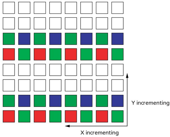
Figure 14: Pixel Readout (x- and y-direction skipping)
