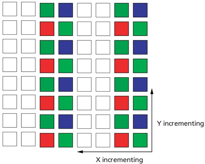
Figure 13: Pixel Readout (y-direction skipping)
