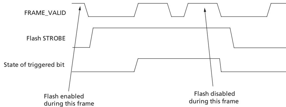
**Figure 20: LED Flash Using Inverted STROBE**
