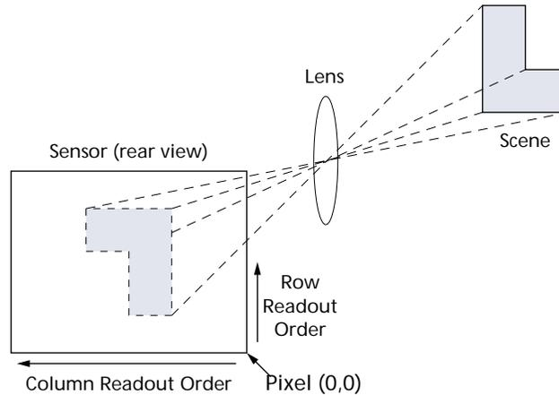
The sensor core supports different readout options to modify the image before it is sent to the IFP. The readout can be limited to a specific window size of the original pixel array.
