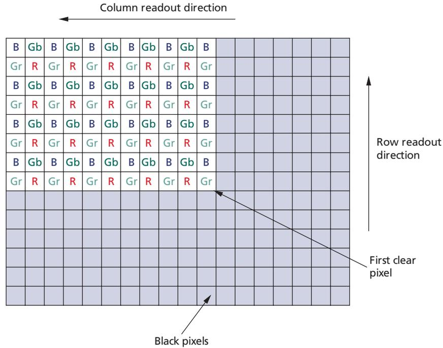
The MT9V113 sensor core pixel array is shown with pixel (0,0) in the bottom right corner, which reflects the actual layout of the array on the die. Figure 7 on page 16 shows the image shown in the sensor during normal operation.
