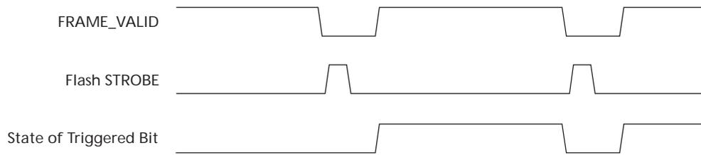
**Figure 19: LED Flash Enabled**
