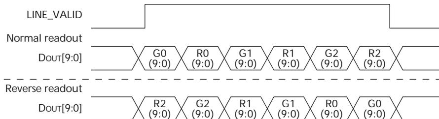
When the sensor is configured to flip the image vertically, the order in which pixel rows are read out is reversed, so that row readout starts from the last row address and ends at the first row address. Figure 9 shows a sequence of 6 rows being read out with normal readout and reverse readout. This change in sensor core output is corrected by the IFP.
