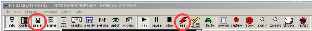
3. Open Preset window, click on "Browse..." and locate the lens correction .ini file. Enable LC by setting R0x3780 bit[15] to "1."
