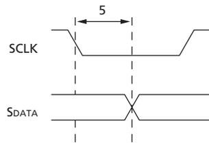
Notes: 1. SDATA is pulled LOW by the sensor or allowed to be pulled HIGH by a pull-up resistor off-chip.
