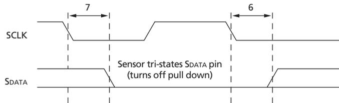
Notes: 1. After a read, the master receiver must pull down SDATA to acknowledge receipt of data bits. When read sequence is complete, the master must generate a no acknowledge by leaving SDATA to float HIGH. On the following cycle, a start or stop bit may be used.
