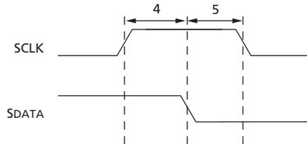
**Figure 39: Serial Host Interface Stop Condition Timing**
