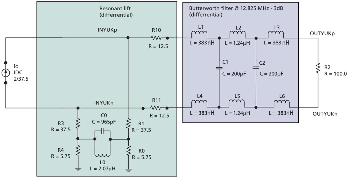
Figure 22: Differential Connection—Grounded Terminations
