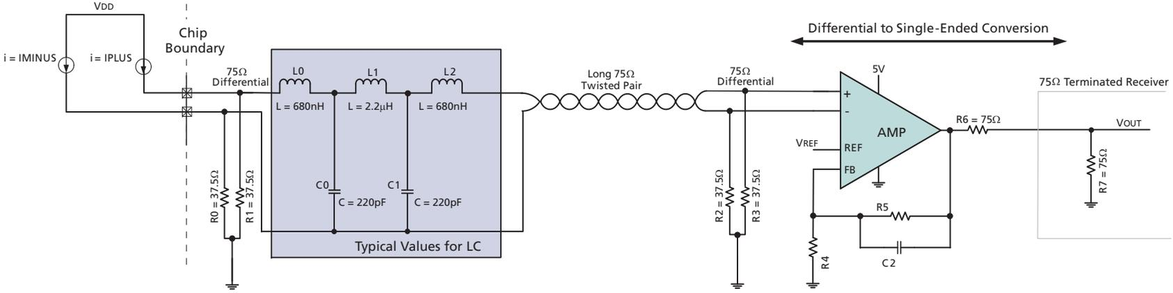
Figure 23: Differential Connection—Floating Termination
