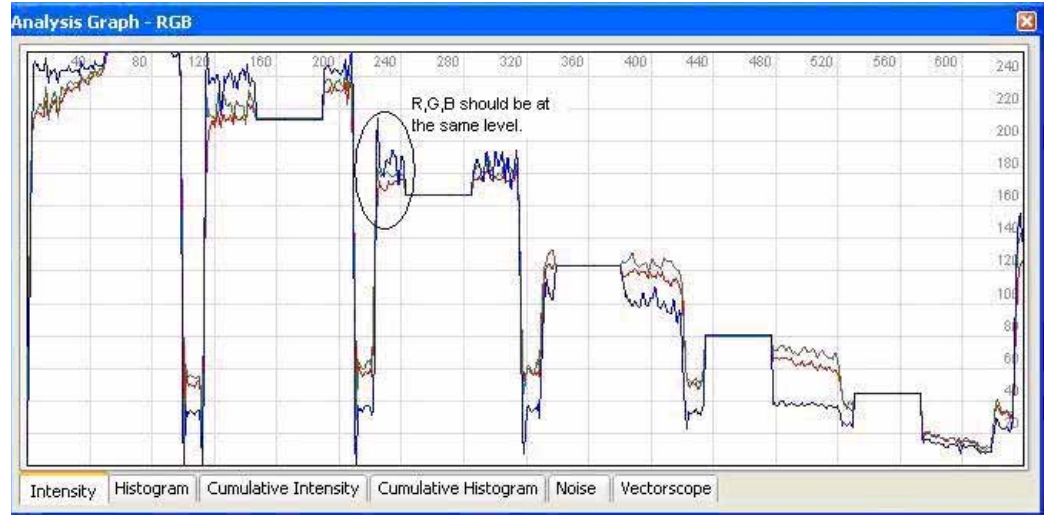
Figure 12: Analysis Graph - RGB Window Showing R,G,B Components of the Macbeth Chart
